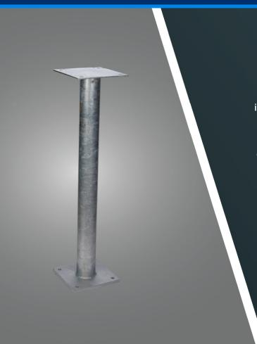
The **BCN-BRKT-4FT** allows the mounting position of medium intensity obstruction lights and strobe flash heads to be raised by four feet. Both the upper and lower mounting plates feature industry standard mounting hole pattern. The four inch pipe is double welded on the top and bottom side of the reinforced base plate. Sturdy galvanized steel construction resists corrosion. Mounting hardware is included.
