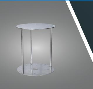
The **BCN-BRKT-DUAL** allows medium intensity obstruction lights and strobe flash heads to be stacked. The bracket can also be used to raise the height of a medium intensity obstruction light or strobe flash head. The mounting areas provide four 0.725" holes on a 13.25" diameter bolt circle.
