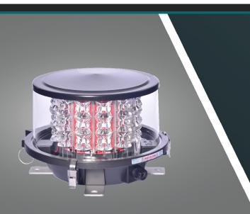
The IFH-1710 utilizes the latest LED technology and advanced optics to achieve a complete red LED wind turbine obstruction lighting system. The IFH-1710 connects with a single cable for ease of installation and meets FAA AC 70/7460-1K requirements. GPS flash synchronization is a standard feature and is configurable to match the flash rates of competitors. The IFH-1710 is designed for long term maintainability with field replaceable circuit boards, photocell and GPS.
