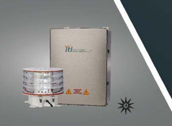
The ILS-3600 Dual LED Lighting System utilizes LED technology and precision optics to provide a low power, low light pollution, dual tower lighting solution. All electronics is accessible at ground level reducing the need for costly tower climbs. The flash head contains only LEDs and a multi-stage surge suppression network. System modularity facilitates maintenance and long term reliability. Low noise design enhances compatibility with 4G/LTE technology.
