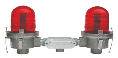
Precision molded Fresnel Optics produce a low ground scatter tower lighting solution. Die cast **aluminum construction** provides a 3/4 inch conduit hub for bottom mounting. Multiple 9kA MOVs and 20kA gas plasma discharge tubes provide robust surge suppression.
