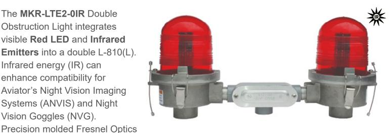
produce a low ground scatter tower lighting solution. Die cast aluminum construction provides a 3/4 inch conduit hub for bottom mounting. Multiple 9kA MOVs and 20kA gas plasma discharge tubes provide robust surge suppression.
