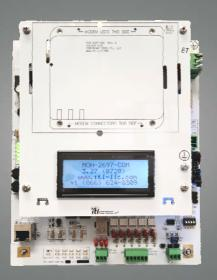
ITL's MON-2697-COM is designed to provide a complete monitoring solution for ITL LED tower lighting systems. The integrated RS232/485 port allows smart monitoring of generators (Generac, Koler, Etc) and automatic transfer switches. The monitoring system's rich set of features is directly applicable to monitoring all aspects of these two LED lighting systems.
