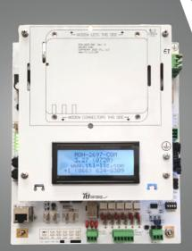
ITL's MON-2697-COM is designed to provide a complete monitoring solution for ITL LED tower lighting systems. The integrated RS232/485 port allows smart monitoring of generators (Generac, Kohler, etc) and automatic transfer switches.
