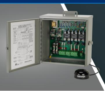
he **RLC-203-GUI Controller** provides wireless flash synchronization for type A-2 AM Tower arrays.
