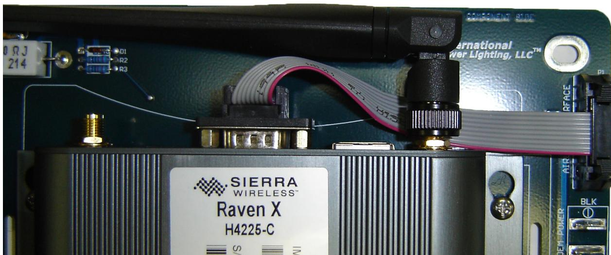
Figure 9: ITL-G930 Wireless Modem Connection
